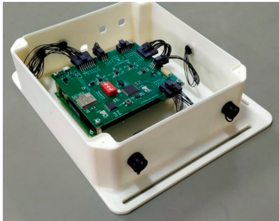
Figure 5. The Remote Monitoring and Control (RMC) system inside its Housing.
